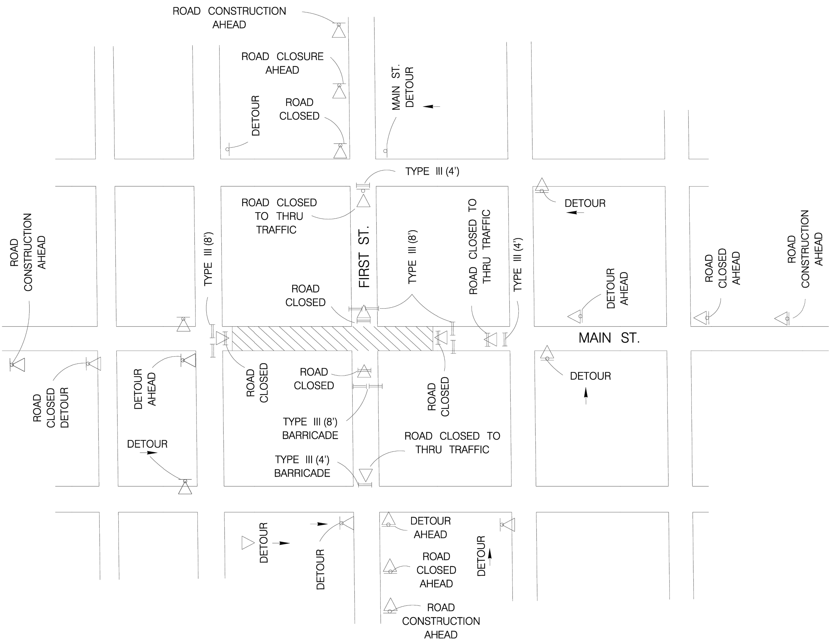
TYPICAL INTERSECTING STREET CLOSURE FOR TWO LANE STREETS
