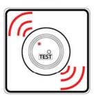
Smoke alarms should be tested once a month by pressing the TEST button.
