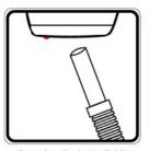
Occasionally dust or lightly vacuum the exterior of the alarm to remove dust and cobwebs.
