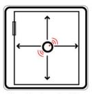
If possible, alarms should be mounted in the center of a ceiling.
