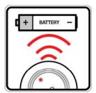
Smoke alarm batteries should be replaced at least once a year. If an alarm "chirps" or beeps to indicate low batteries, they should be replaced immediately.
