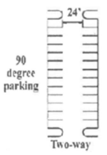
Variance #05 Parking angle in conjunction with two way traffic dictates the minimum required drive aisle width
