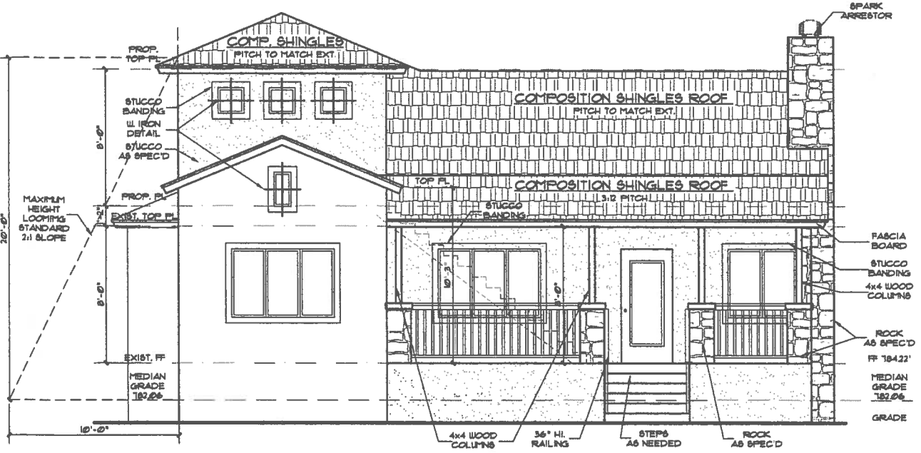
PROPOSED FRONT ELEVATION SCALE: 1/8" = 1'-0"
